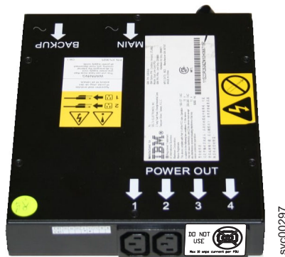
Figure 47. Photo of the redundant ac-power switch
