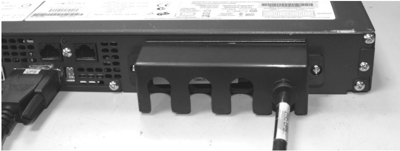
Figure 318. The 2145 UPS-1U cable retention bracket connected to the 2145 UPS-1U
