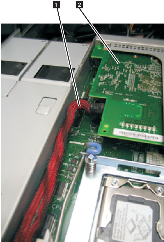
Figure 199. High-speed SAS adapter assembly and high-speed SAS cable in the SAN Volume Controller 2145-CG8 or 2145-CF8
