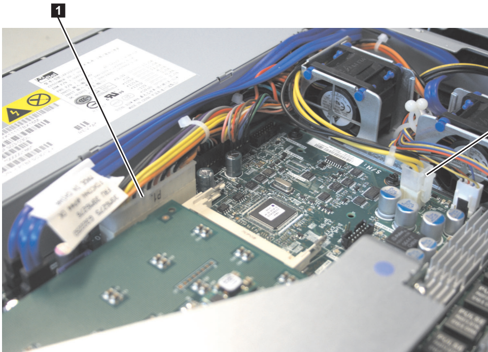
Figure 156. SATA connectors on the SAN Volume Controller 2145-8A4 system board
