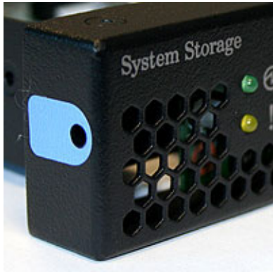
Figure 78. SAN Volume Controller 2145-8G4 service controller release button
