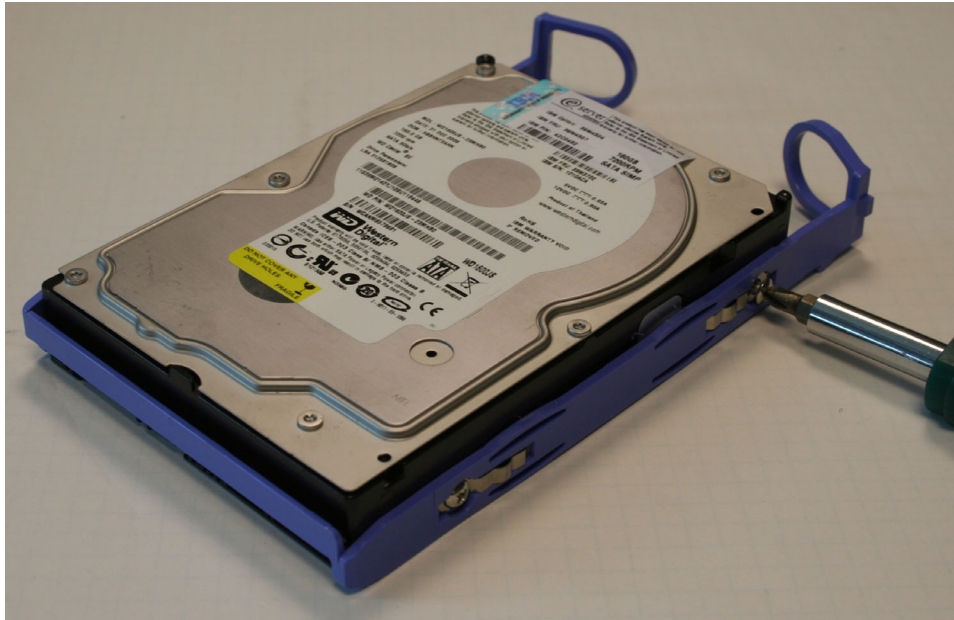
Figure 107. Attaching the rails assembly to the SATA disk drive for the SAN Volume Controller 2145-8A4 and the SAN Volume Controller 2145-8G4
