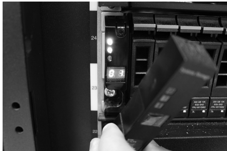
Figure 10. Removing the enclosure end cap
