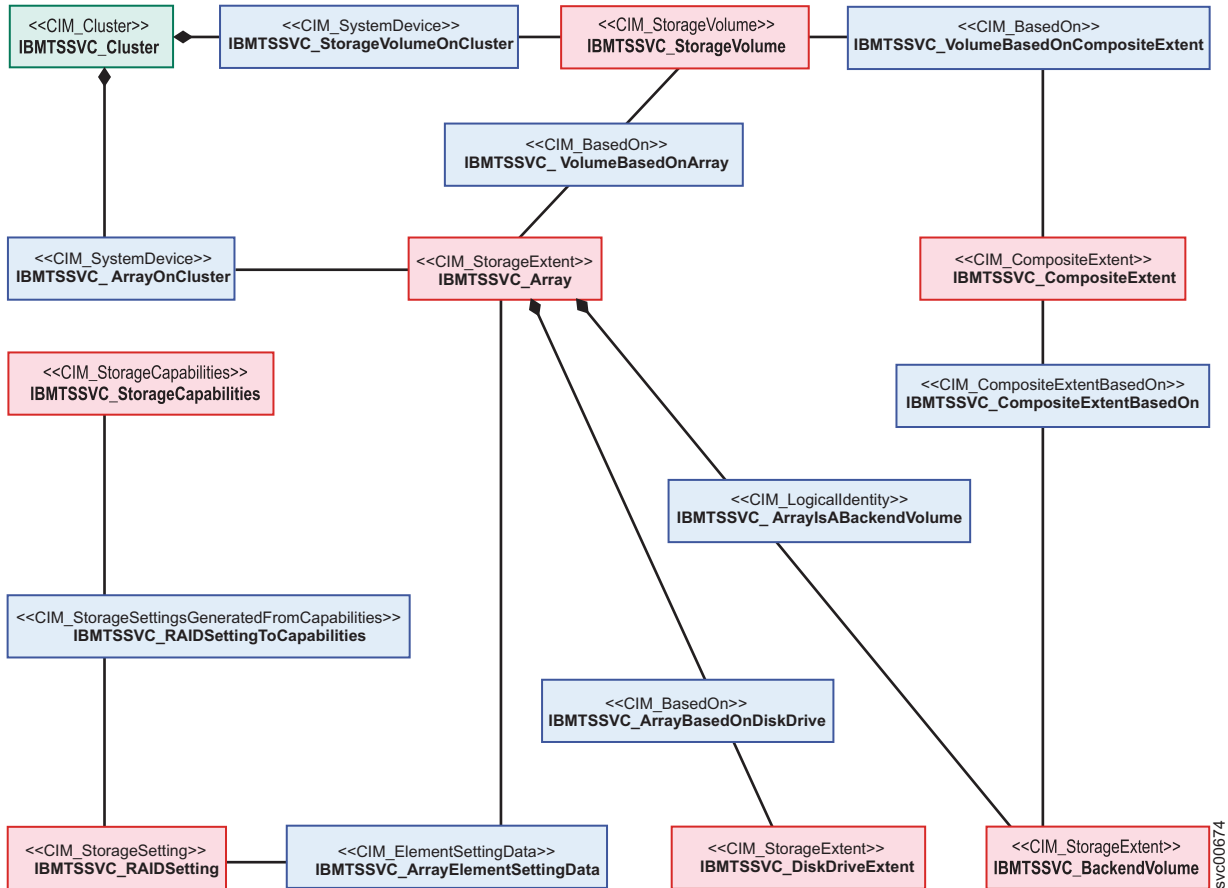
Figure 7. RAID support for block services
