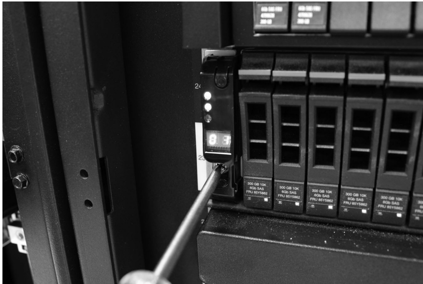
Figure 11. Securing an enclosure to a rack cabinet
