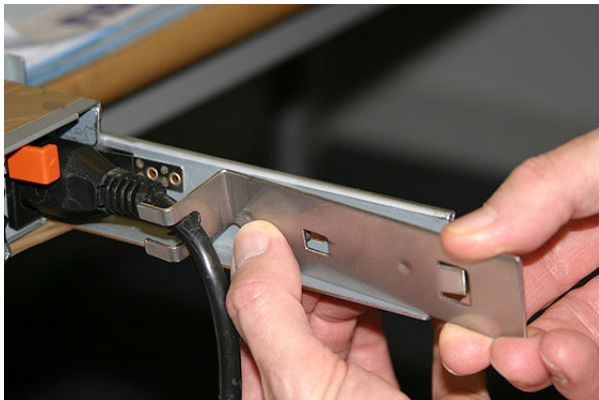
Figure 31. Attaching the cable retention bracket to the SAN Volume Controller 2145-8F4 power cable
