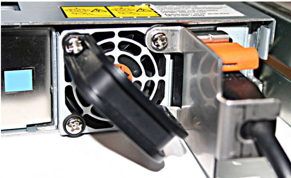
Figure 22. The SAN Volume Controller 2145-8G4 with the cable-retention bracket attached
