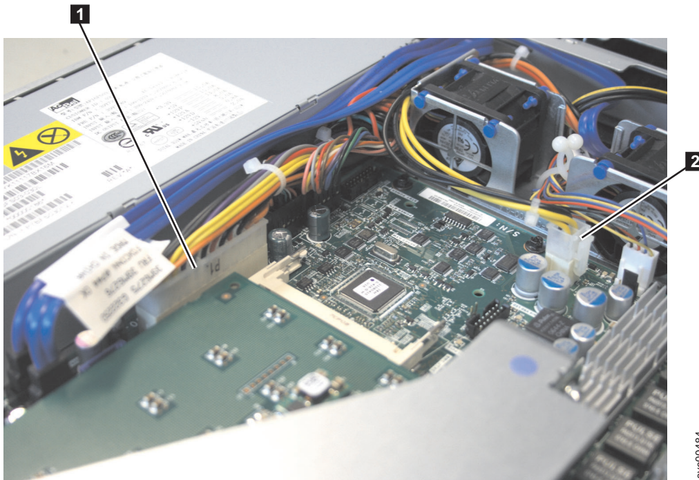
Figure 156. SATA connectors on the SAN Volume Controller 2145-8A4 system board
