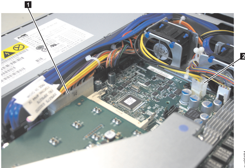
Figure 147. SATA connectors on the SAN Volume Controller 2145-8A4 system board
