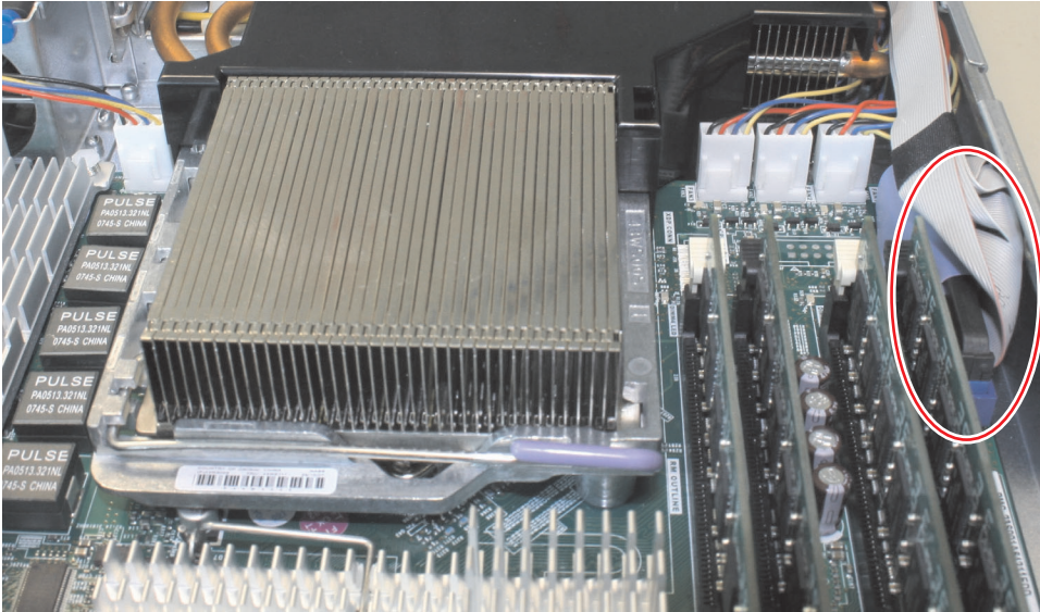
Figure 278. The IDE connector on the SAN Volume Controller 2145-8A4 system board
