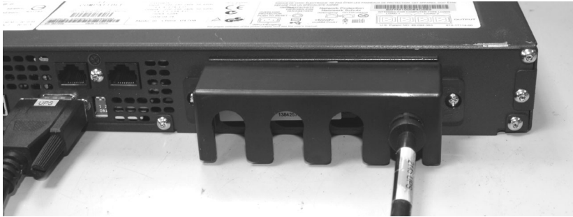
Figure 319. The 2145 UPS-1U cable retention bracket connected to the 2145 UPS-1U
