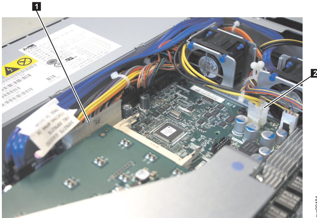
Figure 158. SATA connectors on the SAN Volume Controller 2145-8A4 system board
