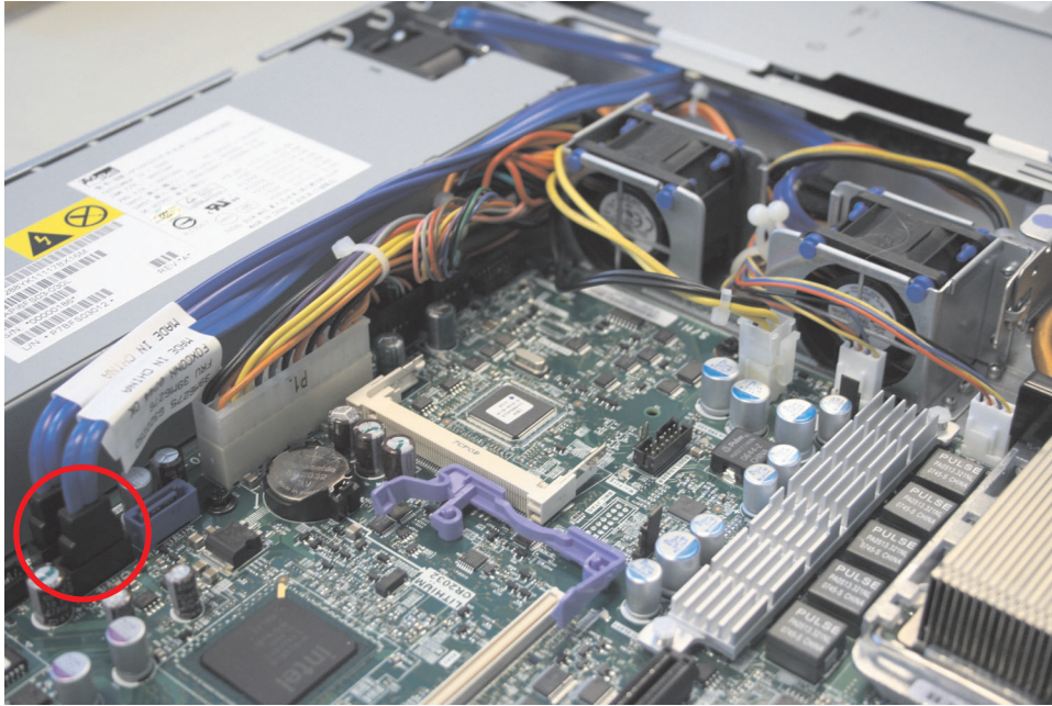
Figure 116. SAN Volume Controller 2145-8A4 SATA cable connectors
