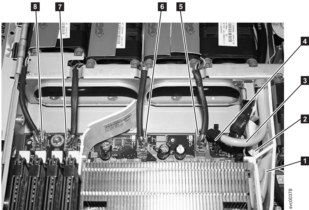
Figure 283. Connectors on the right front side of the SAN Volume Controller 2145-8G4 system board
