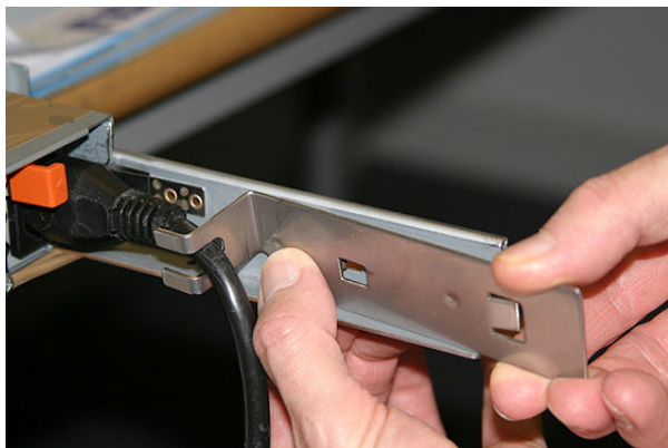
Figure 32. Attaching the cable retention bracket to the SAN Volume Controller 2145-8F4 power cable
