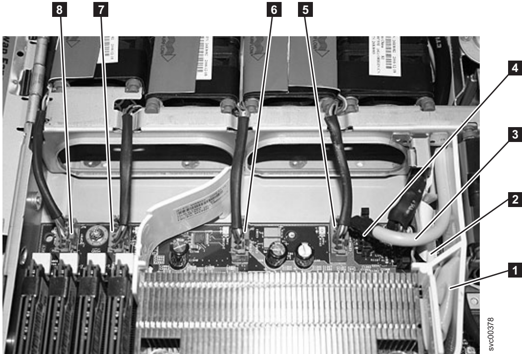
Figure 300. Connectors on the right front side of the SAN Volume Controller 2145-8G4 system board
