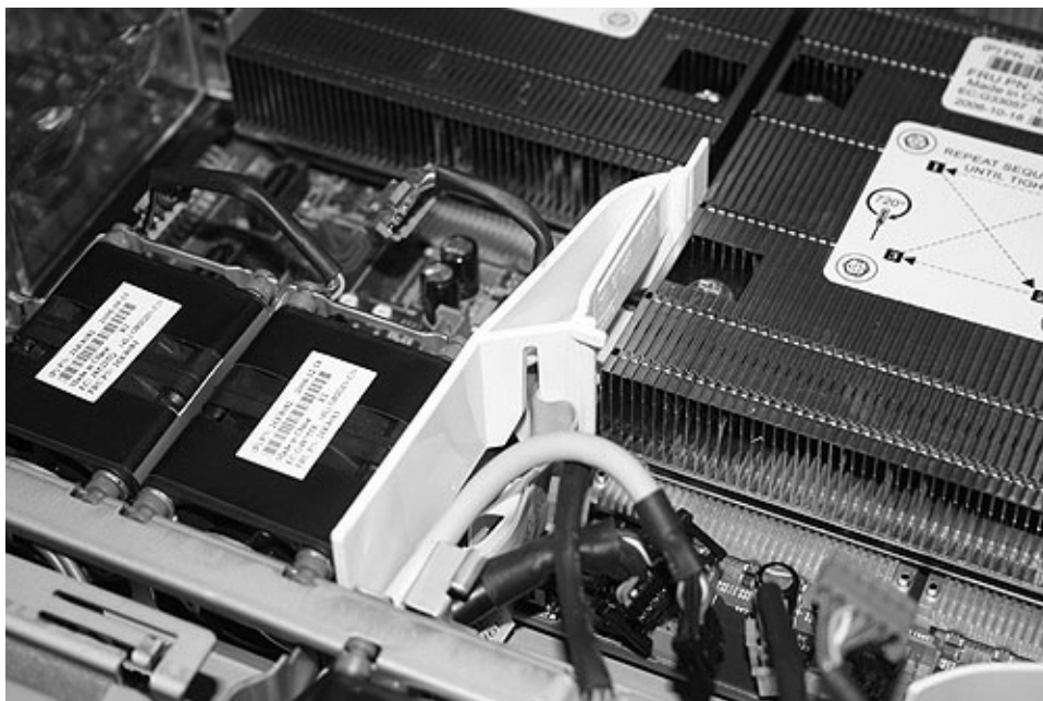
Figure 282. Left air baffle on the SAN Volume Controller 2145-8G4
