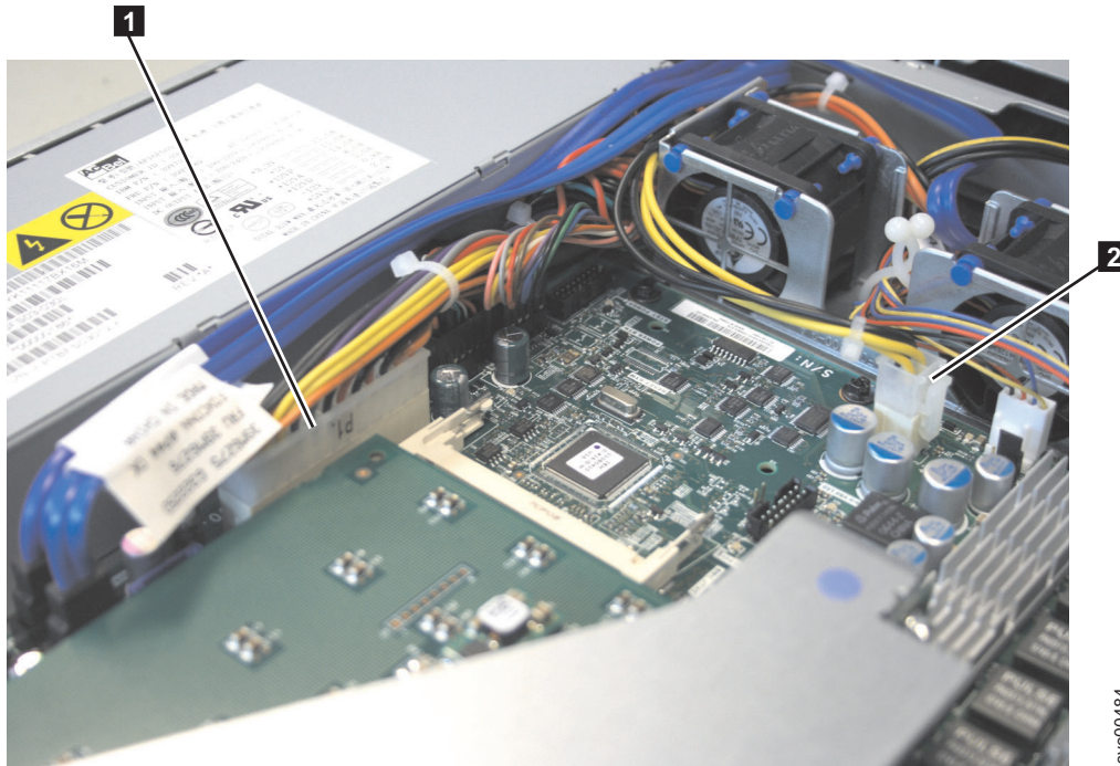
Figure 149. SATA connectors on the SAN Volume Controller 2145-8A4 system board
