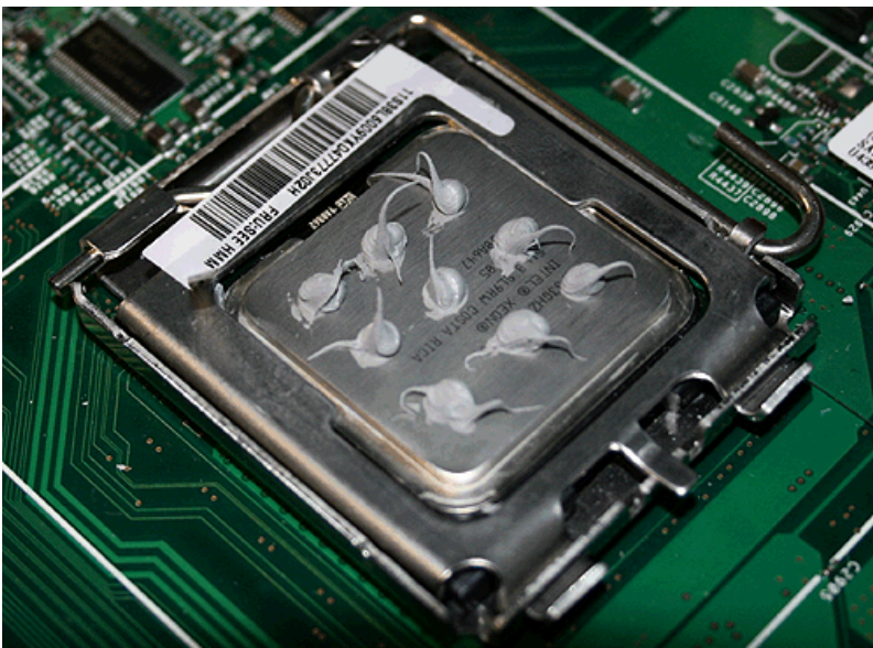
Figure 299. Complete set of nine thermal grease dots on the microprocessor
