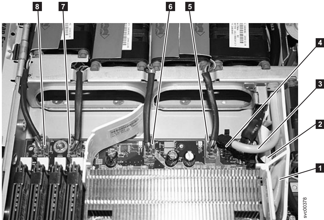
Figure 301. Connectors on the right front side of the SAN Volume Controller 2145-8G4 system board
