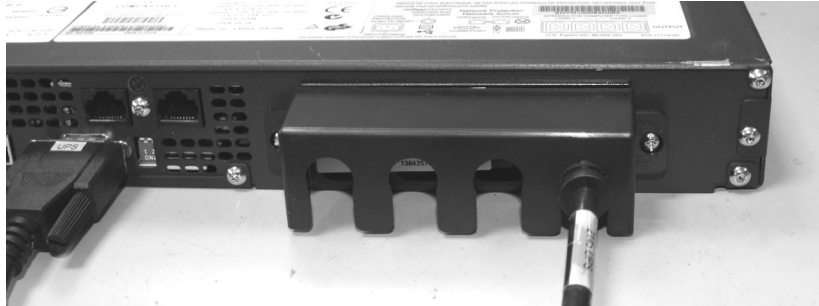
Figure 308. 2145 UPS-1U power cable-retention bracket
