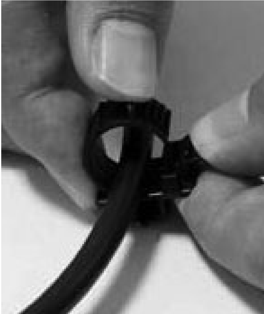
Figure 31. Unlocking the cable retention bracket
