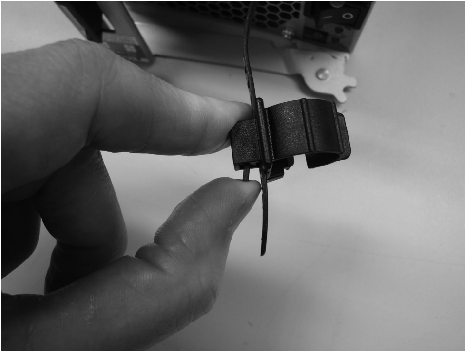
Figure 32. Pressing the lever to slide the cable retention bracket.
