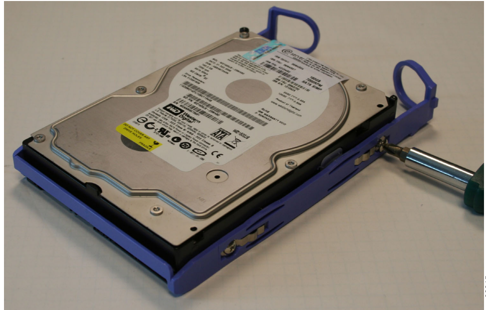
Figure 165. Attaching the rails assembly to the SAN Volume Controller 2145-8G4 SATA disk drive
