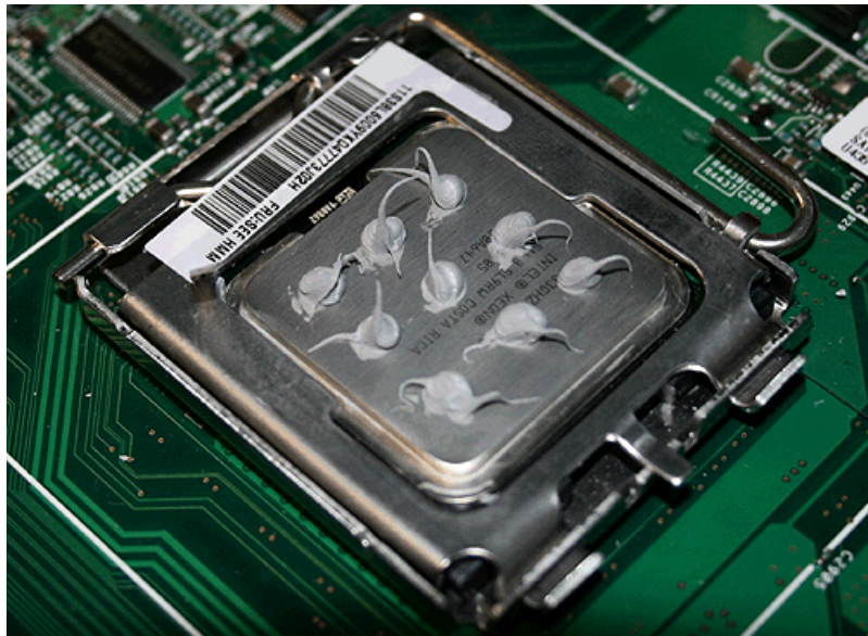
Figure 248. Complete set of nine thermal grease dots on the microprocessor
