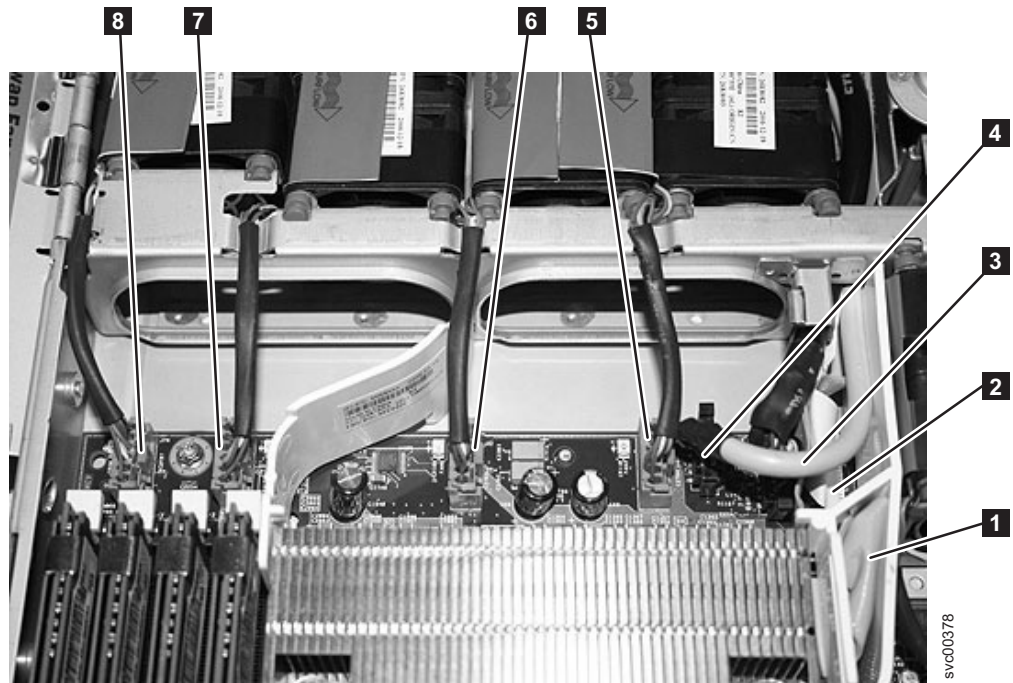
Figure 236. Connectors on the right front side of the SAN Volume Controller 2145-8G4 system board
