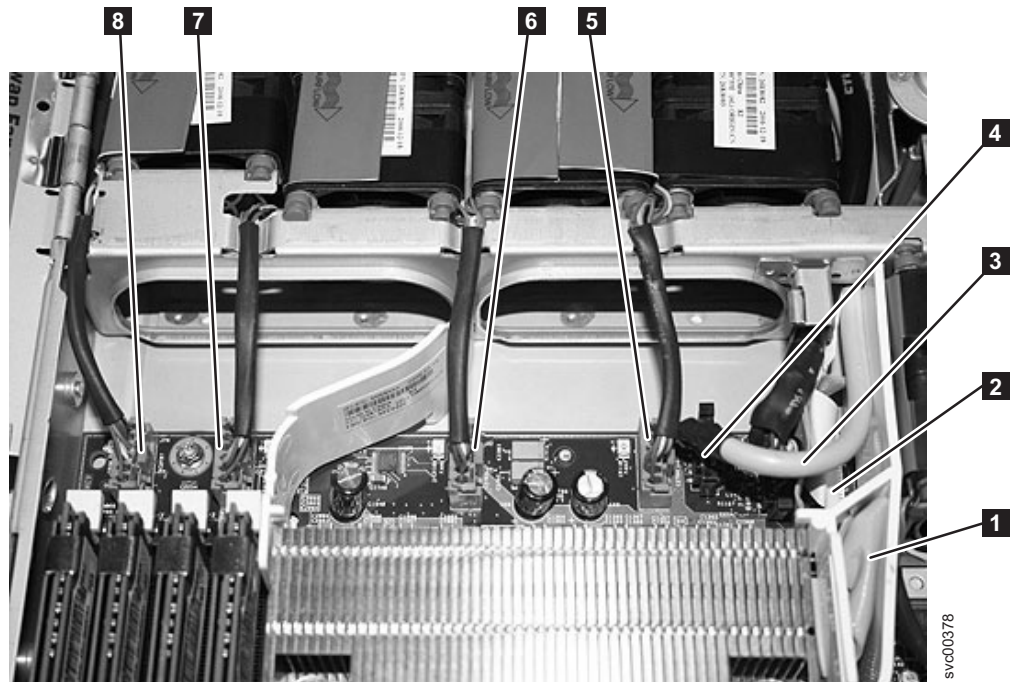
Figure 250. Connectors on the right front side of the SAN Volume Controller 2145-8G4 system board
