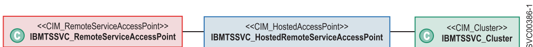
Figure 5. High-level overview of the access point subprofile of the CIM Agent for the SAN Volume Controller.
