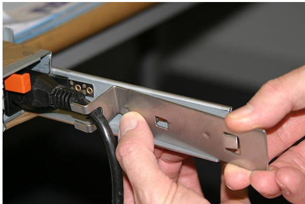
Figure 44. Attaching the cable retention bracket to the SAN Volume Controller 2145-8F4 power cable
