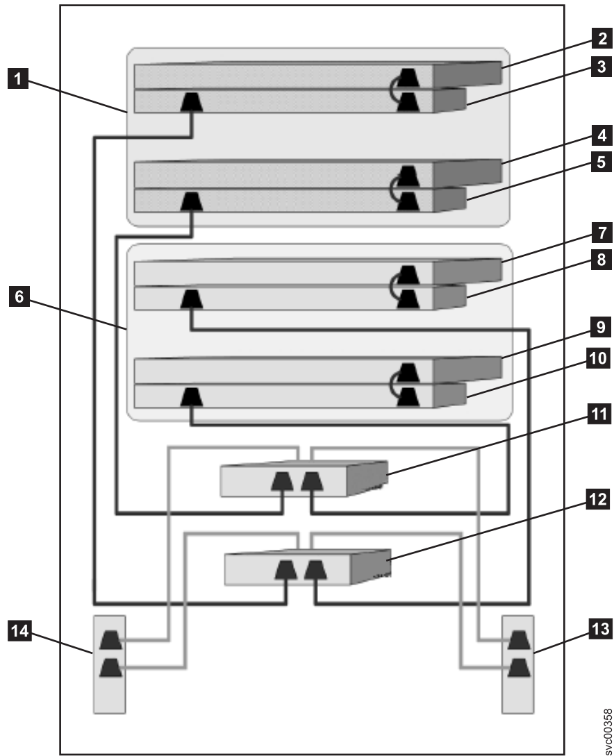
Figure 16. A four-node SAN Volume Controller cluster with the redundant ac-power switch feature
