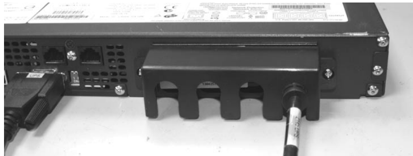
Figure 37. 2145 UPS-1U power cable-retention bracket
