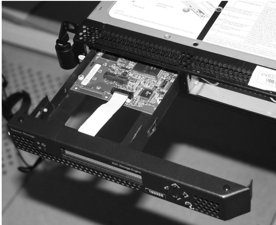
Figure 62. Removing the service controller from the SAN Volume Controller 2145-8G4
