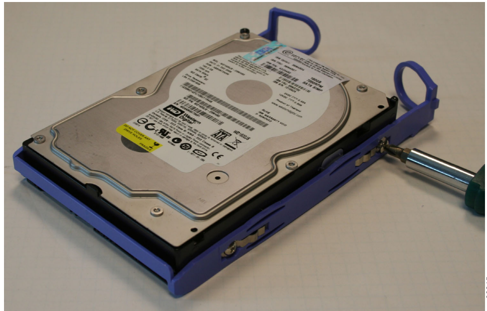
Figure 90. Attaching the rails assembly to the SATA disk drive for the SAN Volume Controller 2145-8A4 and the SAN Volume Controller 2145-8G4
