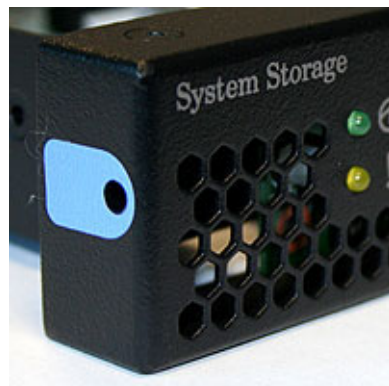
Figure 61. SAN Volume Controller 2145-8G4 service controller release button
