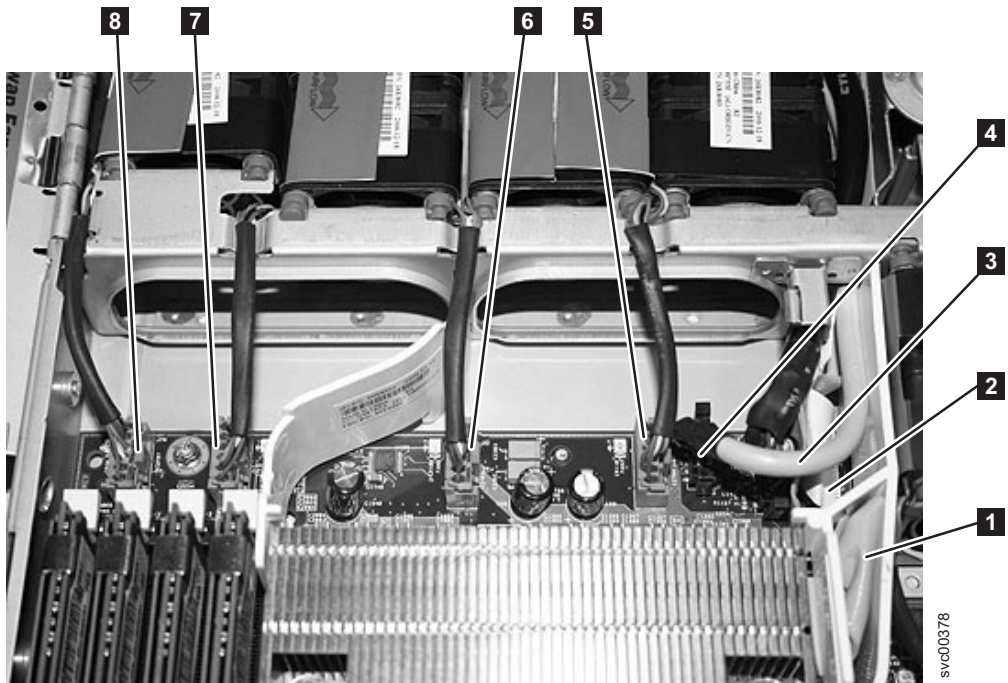
Figure 200. Connectors on the right front side of the SAN Volume Controller 2145-8G4 system board
