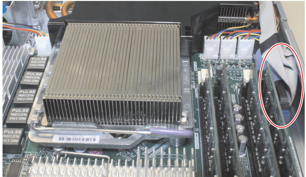
Figure 195. The IDE connector on the SAN Volume Controller 2145-8A4 system board
