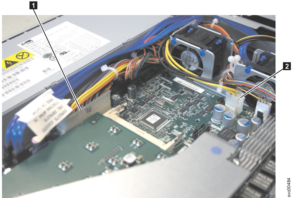
Figure 127. SATA connectors on the SAN Volume Controller 2145-8A4 system board
