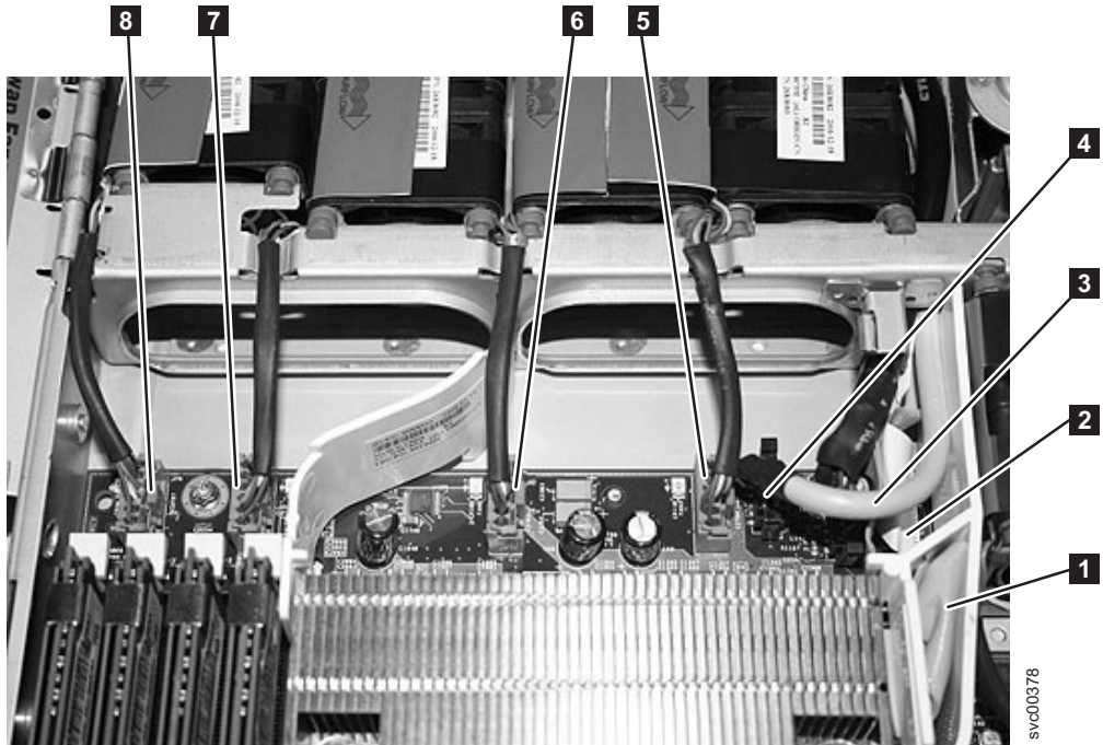
Figure 216. Connectors on the right front side of the SAN Volume Controller 2145-8G4 system board
