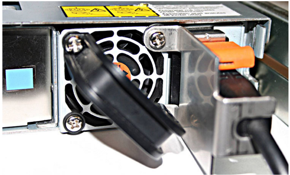
Figure 12. The SAN Volume Controller 2145-8G4 with the cable retention bracket attached
