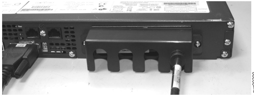
Figure 237. The 2145 UPS-1U cable retention bracket connected to the 2145 UPS-1U
