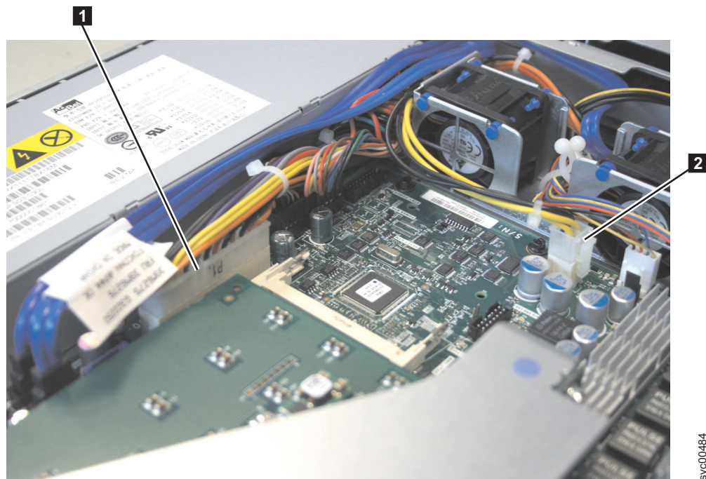
Figure 119. SATA connectors on the SAN Volume Controller 2145-8A4 system board
