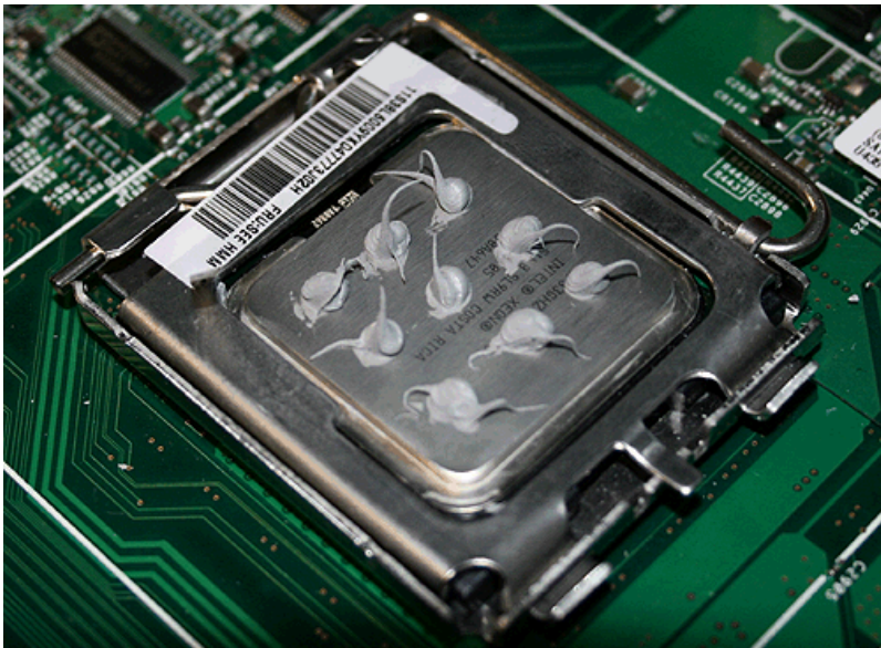
Figure 214. Complete set of nine thermal grease dots on the microprocessor
