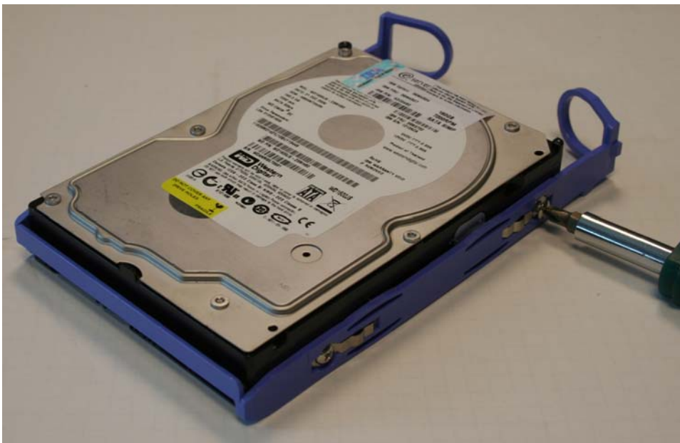
Figure 126. Attaching the rails assembly to the SAN Volume Controller 2145-8G4 SATA disk drive
