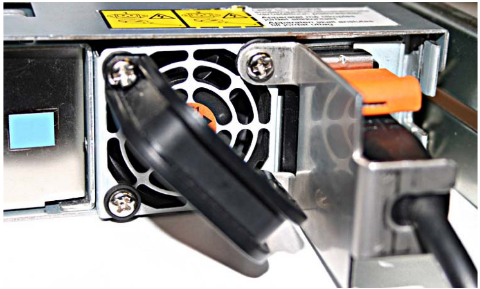
Figure 33. The SAN Volume Controller 2145-8G4 with cable retention bracket option A attached
