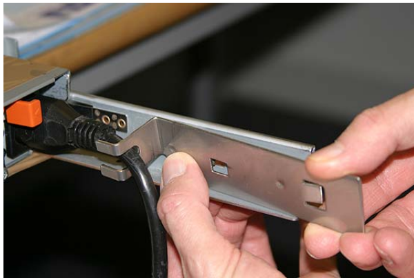
Figure 66. Attaching the cable retention bracket to the SAN Volume Controller 2145-8F4 power cable
