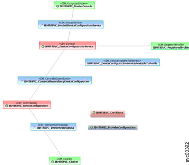
Figure 8. Class diagram of device configuration instances
