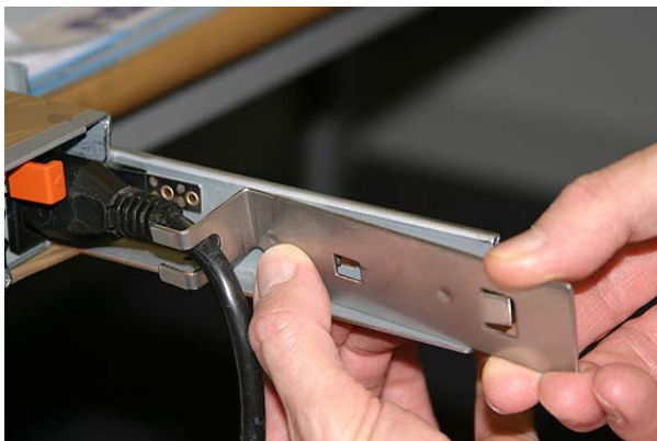
Figure 46. Attaching the cable retention bracket to the SAN Volume Controller 2145-8F4 power cable
