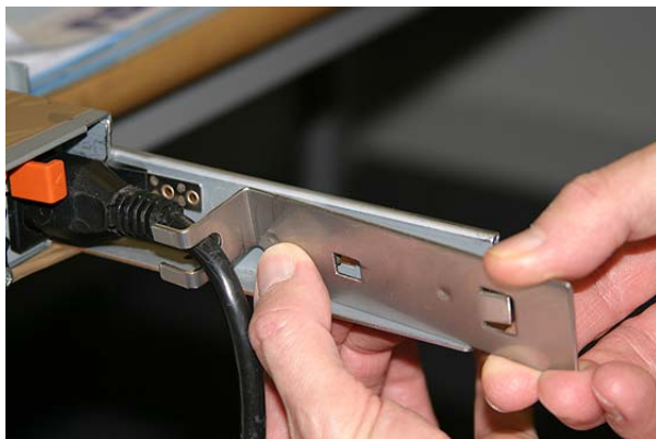
Figure 13. Attaching the cable retention bracket to the SAN Volume Controller 2145-8F4 power cable
