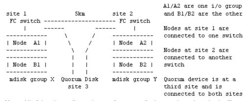
**Note:** All of the above discussion applies to a split cluster where there is significant optical distance between the nodes within a single cluster. Long distance (up to 10 km) connection of remote hosts or remote controllers are supported in an SVC cluster, as the issues of quorum disk and inter IO group links mentioned above are not relevant. Thus, the following configuration is acceptable:
