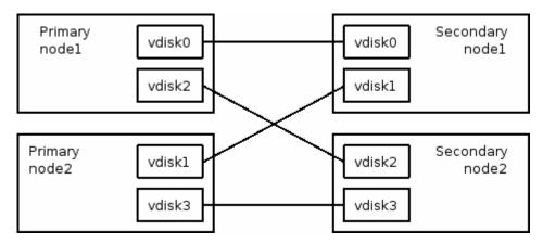
For a configuration that has more than one IO group on either cluster, there are many more primary-secondary node combinations that must be considered when balancing the load.
