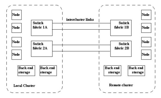
This contains two redundant fabrics. Part of each fabric exists at the local and remote cluster. There is no direct connection between the two fabrics.
