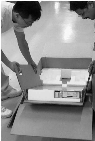
Figure 16. Sliding the uninterruptible power supply to the end of the carton.
