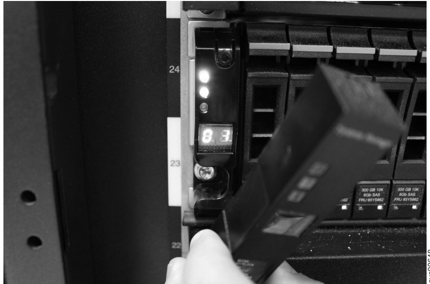
Figure 22. Removing the enclosure end cap
