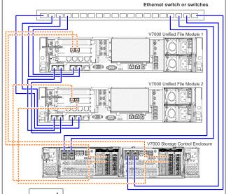
Note that in the default configuration, A Ethernet connections on each Storwize V7000 Unified file module are bonded so each pair of cables and must be plugged into the same Ethernet switch.
