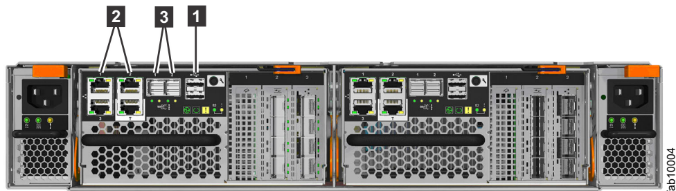
Figure 7. Data ports in the rear of the Storwize V7000 Gen2 control enclosure (2076-524)
