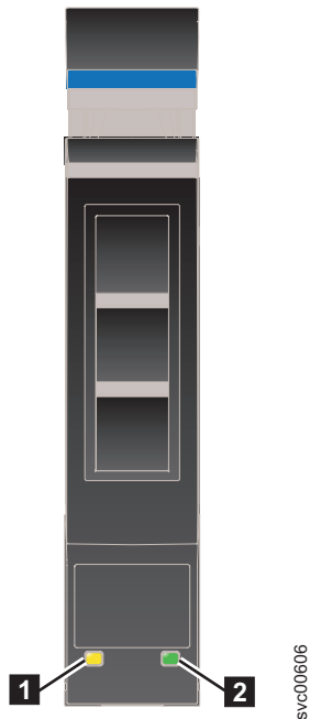
Figure 4. LED indicators on a single 2.5" drive
