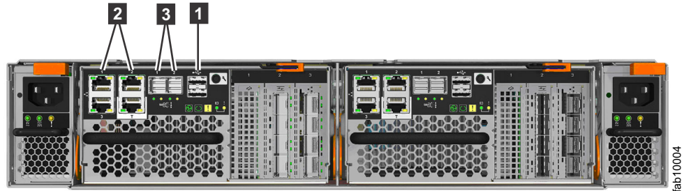
Figure 5. Data ports in the rear of the Storwize V7000 Gen2 control enclosure
