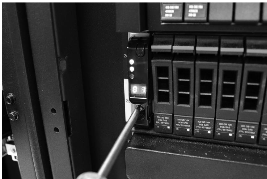
Figure 25. Securing an enclosure to a rack cabinet
