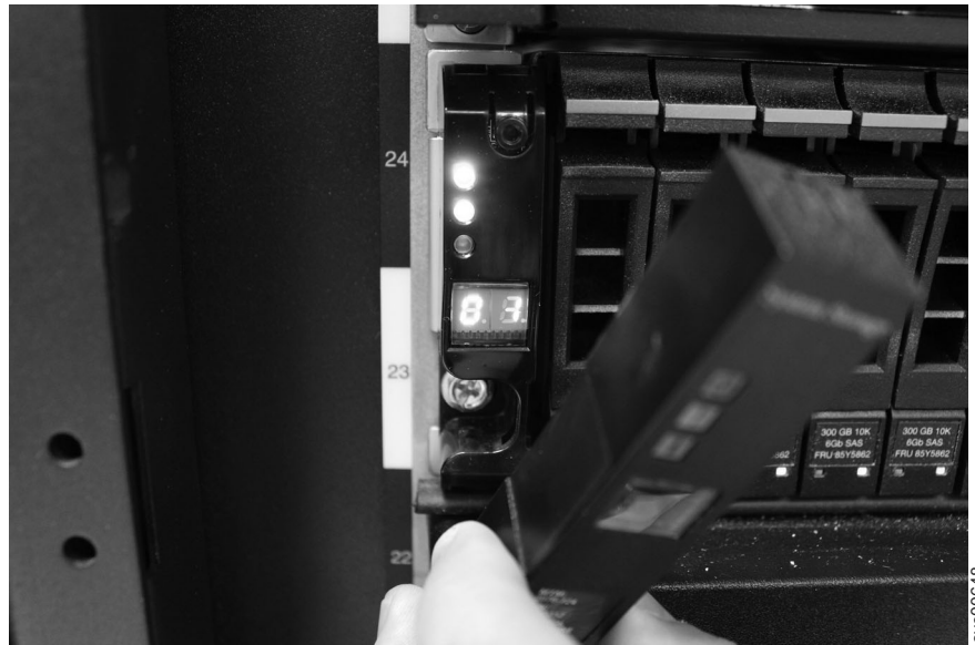
Figure 16. Removing the enclosure end cap
