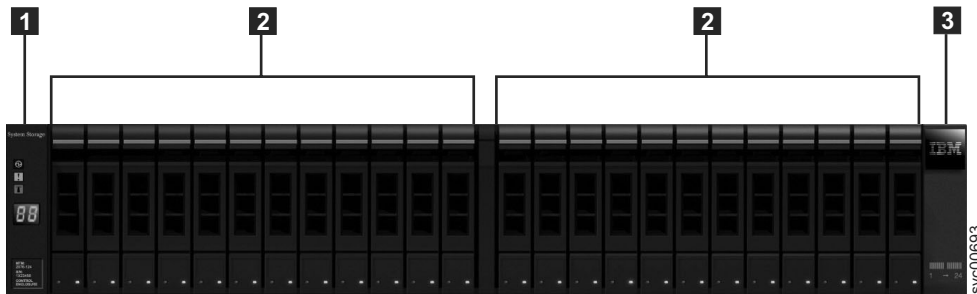
Figure 43. 24 drives and two end caps
