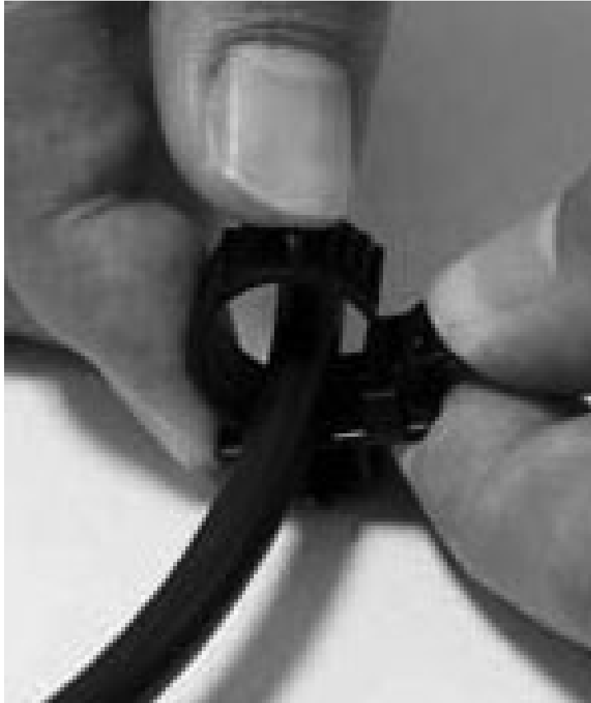
Figure 42. Unlocking the cable retention bracket
