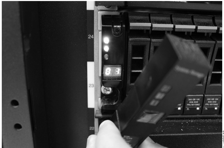
Figure 17. Removing the enclosure end cap
