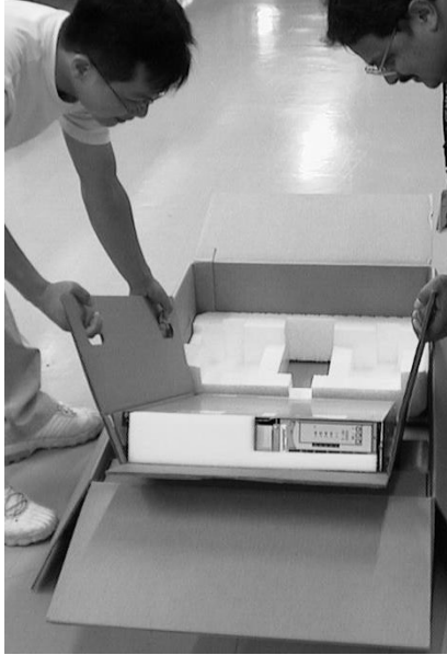
Figure 21. Sliding the uninterruptible power supply to the end of the carton
