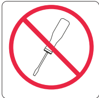
Figure 11. No user access label for the uninterruptible power supply
