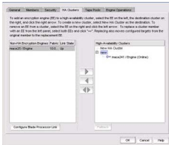
FIGURE 368 Encryption Group Properties dialog box - HA Clusters tab
