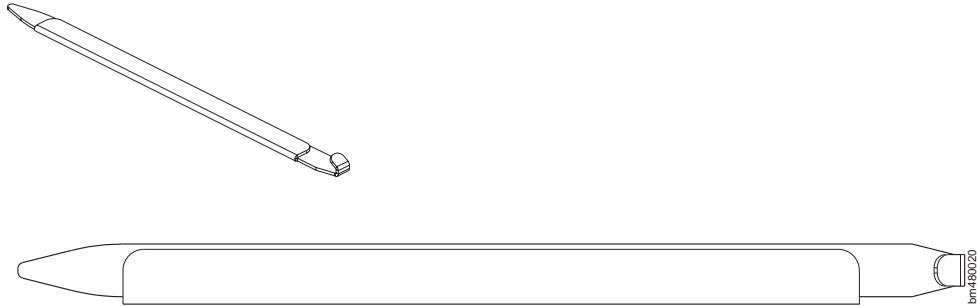
Figure 34. SFP extraction tool
