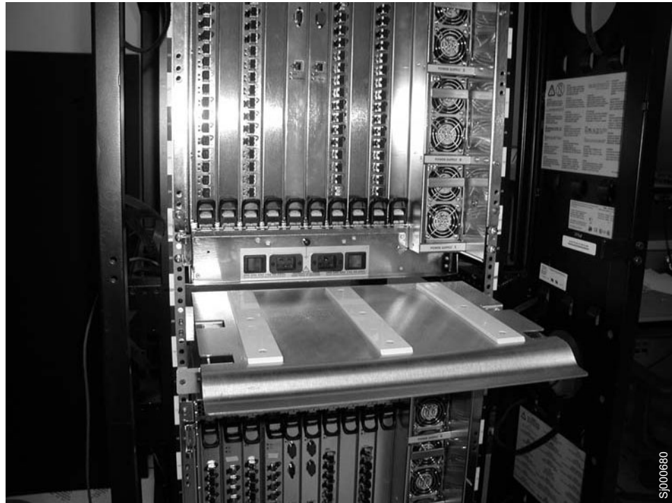
Figure 8. Locking the shelf into position
