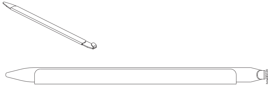
Figure 37. Optical transceiver (SFP+) extraction tool
