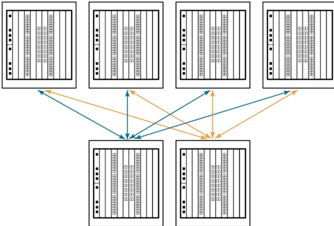
Figure 42. IBM SAN Director core-edge ICL topology
