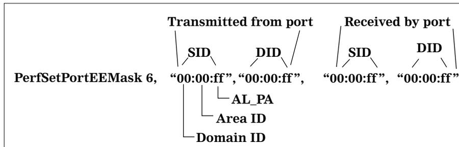
Figure 87. Mask positions for end-to-end monitors
