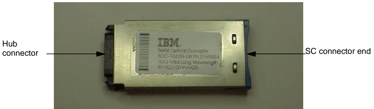
Figure 3. LWL fiber-optic GBIC module (part number and labeling will vary)
