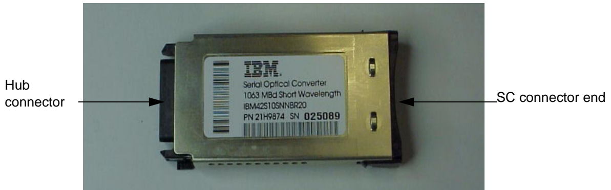
Figure 2. SWL fiber-optic GBIC module (part number and labeling vary)
