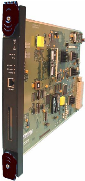
Figure 7. TCM Control Module
