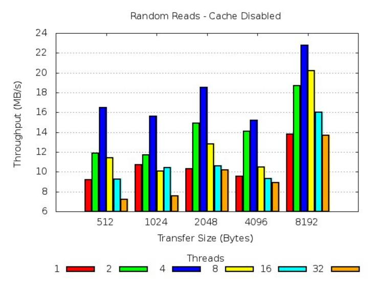
This diagram describes how the random RETRIEVE data throughput rate (MB/sec) was affected as the file transfer size of the objects being retrieved from the DR550 increased and the number of RETRIEVE application threads also successively increased.
