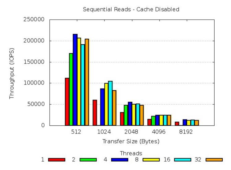
The diagram above shows how a sustained, sequential RETRIEVE data throughput rate (IO's/sec) was affected as the file transfer size of the objects being retrieved from the DR550 increased and the number of RETRIEVE application threads were successively increased.
