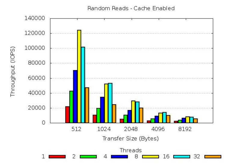
This diagram again describes how the random RETRIEVE data throughput rate (IO's/sec) was affected as the file transfer size of the objects being retrieved from the DR550 increased and the number of RETRIEVE application threads were successively increased.
