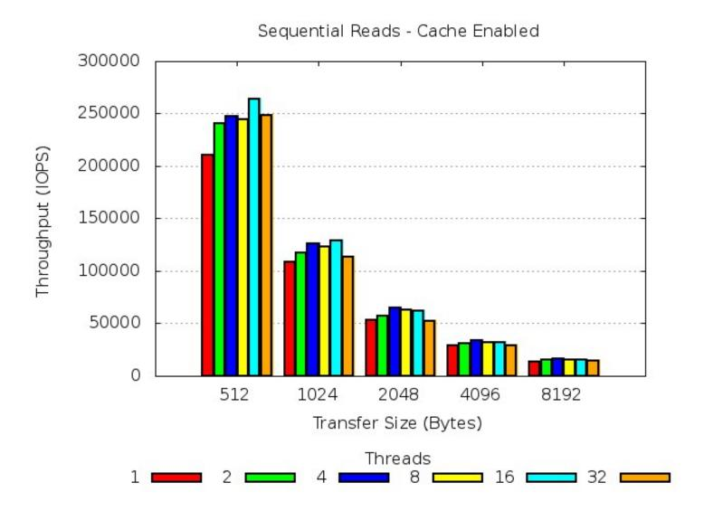
This diagram again describes how a sustained, sequential RETRIEVE data throughput rate (IO's/sec) was affected as the file transfer size of the objects being retrieved from the DR550 increased and the number of RETRIEVE application threads were successively increased.
