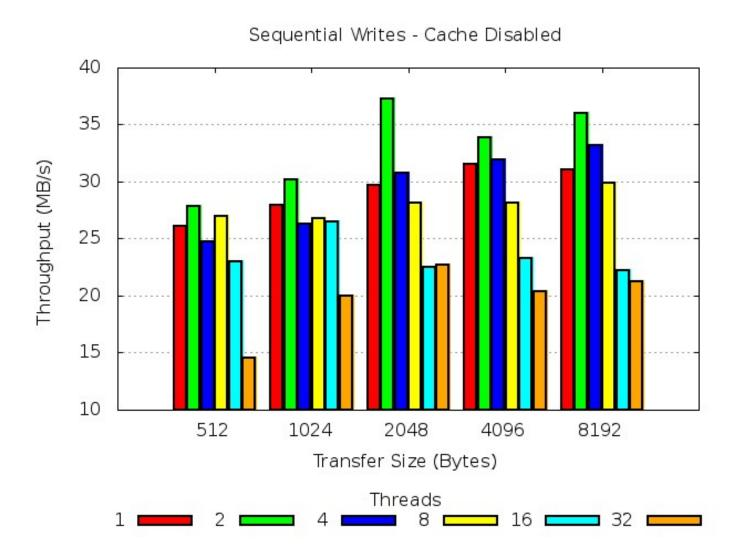
This diagram shows how a sustained sequential, ARCHIVE data throughput rate (MB/sec) was affected as the file transfer size of the objects being written to the DR550 increased and the number of ARCHIVE application threads also successively increased.
