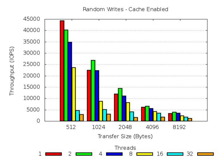
This diagram shows how the ARCHIVE data throughput rate (IO's/sec) was affected as the file transfer size of the objects being written to the DR550 increased and the number of ARCHIVE application threads were also successively increased.
