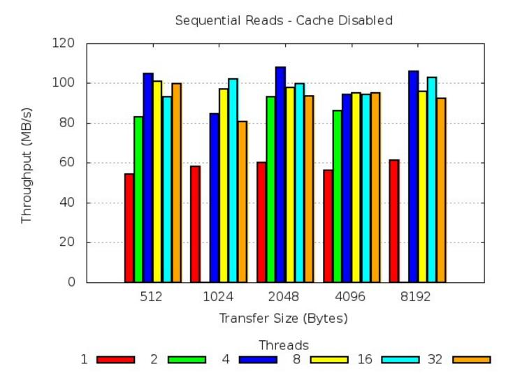
This diagram describes how a sustained, sequential RETRIEVE data throughput rate (MB/sec) was affected as the file transfer size of the objects being retrieved from the DR550 increased and the number of RETRIEVE application threads also successively increased.
