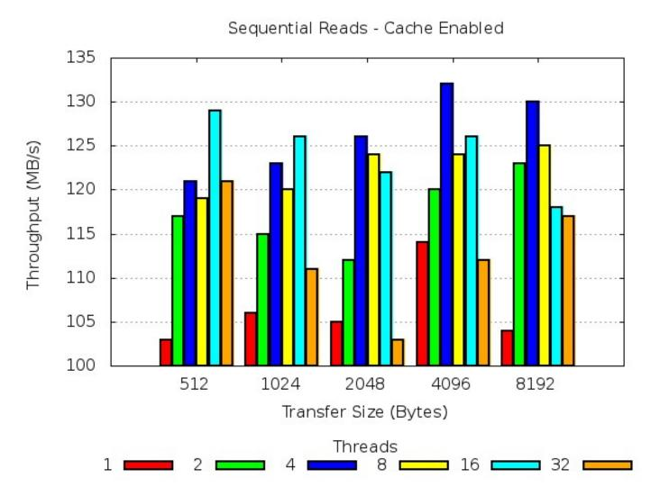
This diagram illustrates how a sequential, sustained RETRIEVE data throughput rate (MB/sec) was affected as the file transfer size of the objects being retrieved from the DR550 increased and the number of RETRIEVE application threads were also successively increased.
