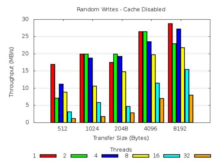
This diagram describes how the ARCHIVE data throughput rate (MB/sec) was affected as the file transfer size of the objects being written to the DR550 increased and the number of ARCHIVE application threads also successively increased.
