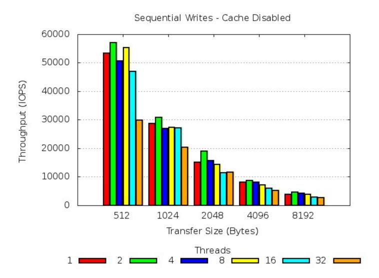
This diagram describes how the sustained, sequential ARCHIVE data throughput rate (IO's/sec) was affected as the file transfer size of the objects being written to the DR550 increased and the number of ARCHIVE application threads also successively increased.
