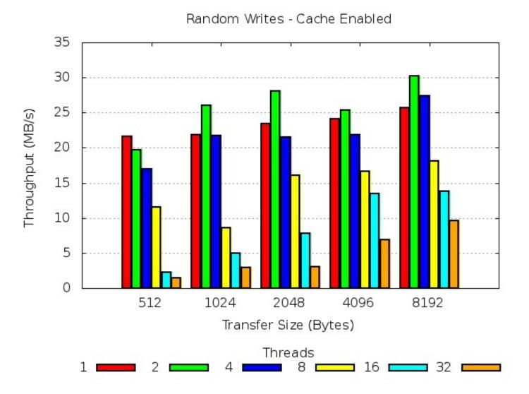
This diagram shows how the ARCHIVE data throughput rate (MB/sec) was affected as the file transfer size of the objects being written to the DR550 increased and the number of ARCHIVE application threads were also successively increased.
