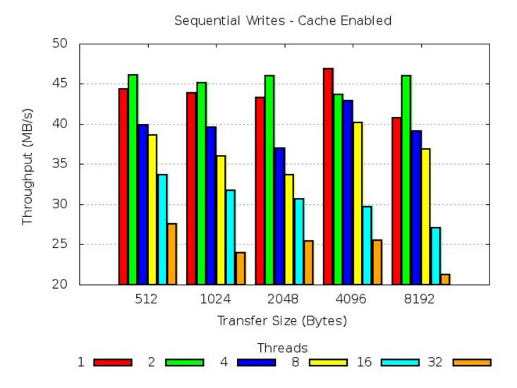
The diagram above shows how the sustained, sequential ARCHIVE data throughput rate (MB/sec) was affected as the file transfer size of the objects being written to the DR550 increased and the number of ARCHIVE application threads were also successively increased.
