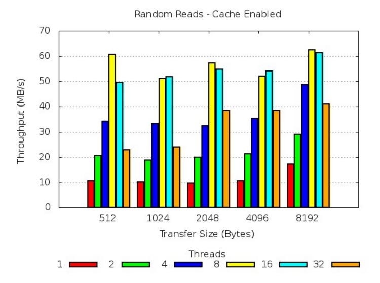
This diagram shows how the random RETRIEVE data throughput rate (MB/sec) was affected as the file transfer size of the objects being retrieved from the DR550 increased and the number of RETRIEVE application threads were also successively increased.
