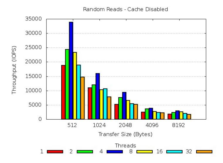
This diagram describes how the random RETRIEVE data throughput rate (IO's/sec) was affected as the file transfer size of the objects being retrieved from the DR550 increased and the number of RETRIEVE application threads were successively increased.
