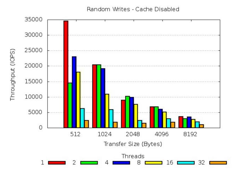
This diagram describes how the ARCHIVE data throughput rate (IO's/sec) was affected as the file transfer size of the objects being written to the DR550 increased and the number of ARCHIVE application threads also successively increased.
