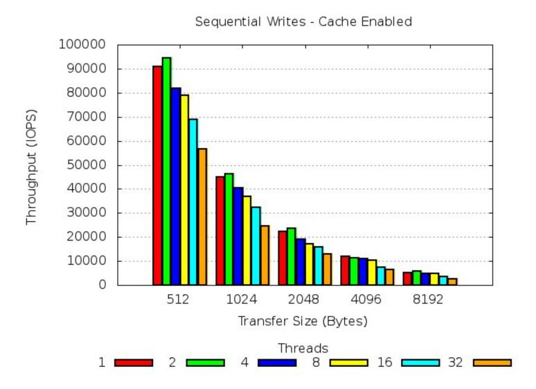
This diagram describes how the sustained, sequential ARCHIVE data throughput rate (IO's/sec) was affected as the file transfer size of the objects being written to the DR550 increased and the number of ARCHIVE application threads were also successively increased.
