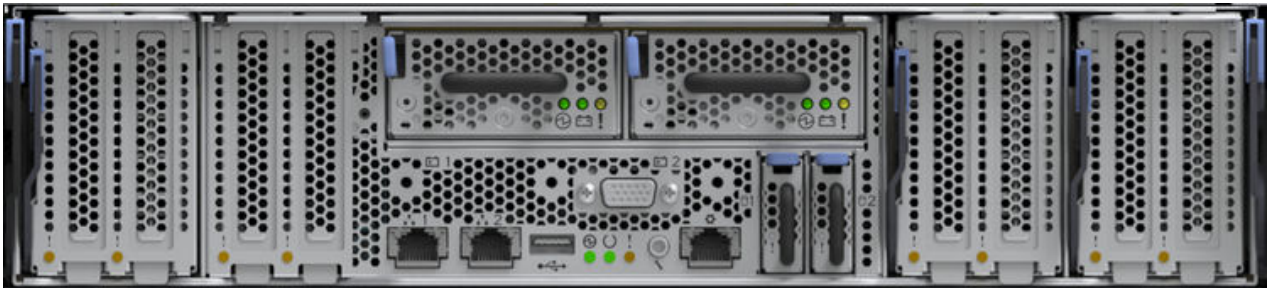
Figure 3. Node canister - Rear view
