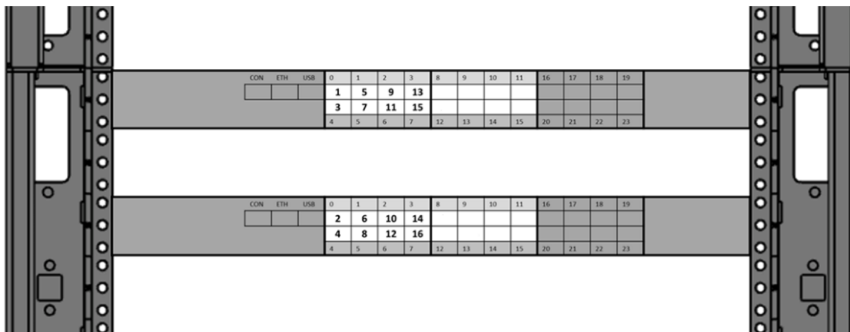
Figure 198. Fibre Channel ports in the IBM SAN24B-6 switches
