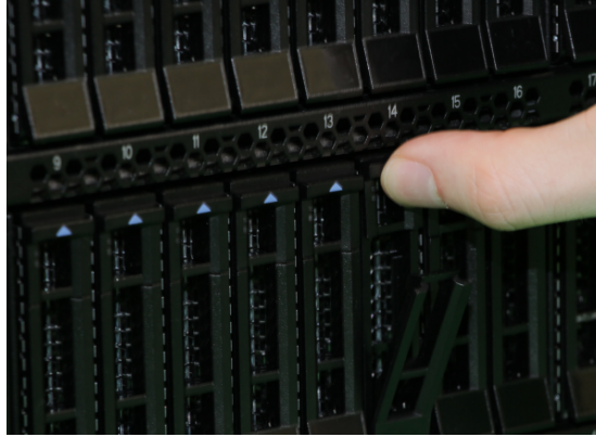
Figure 72. Unlocking the drive and release latch
