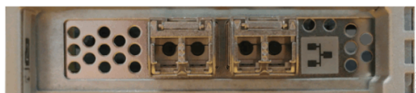
Figure 186. Dual-port 25 Gbps Ethernet host interface adapter ports and LEDs (iWARP)
