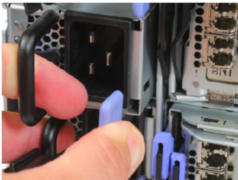
Figure 78. Removing the power supply unit
