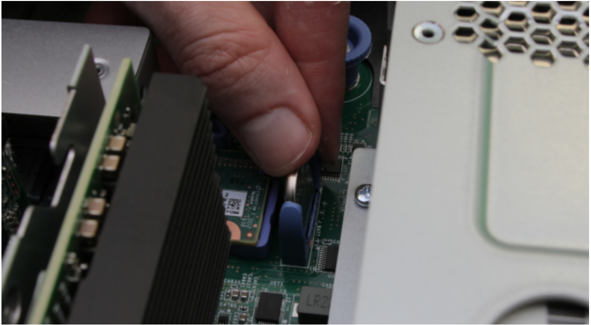
Figure 85. Replacing a CMOS battery
