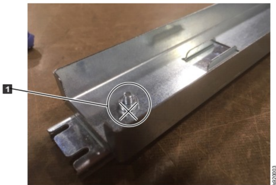
Figure 249. Incorrect screw length
