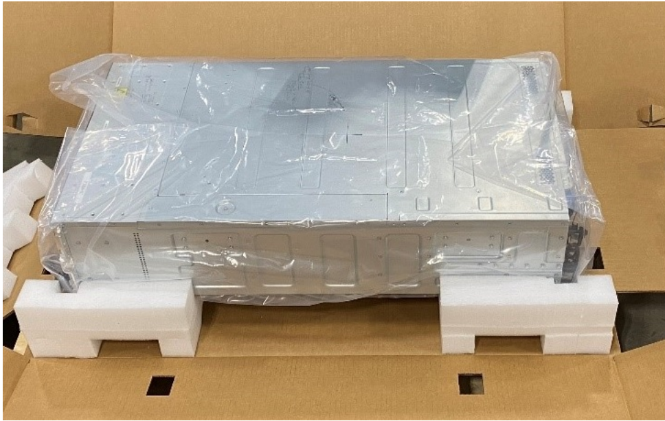
Figure 27. Foam removal from enclosure
