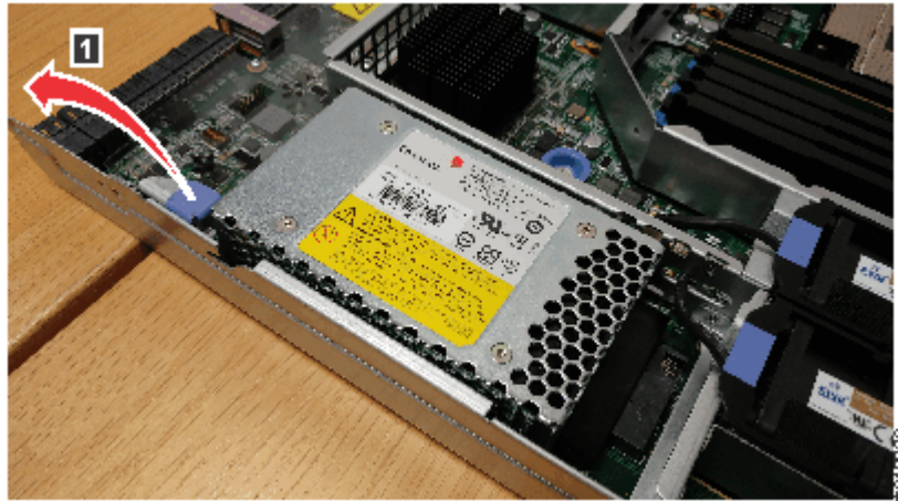
Figure 74. Lifting the latch of the node battery
