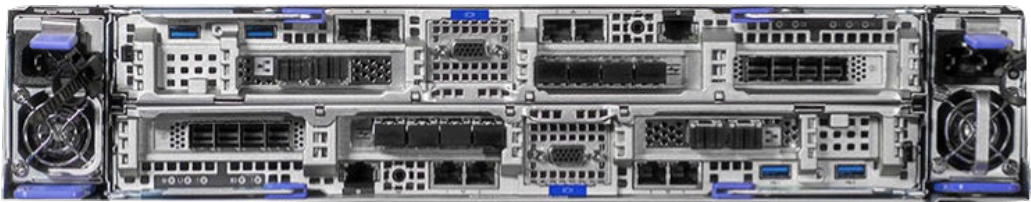
Figure 2. Rear view of the control enclosure
