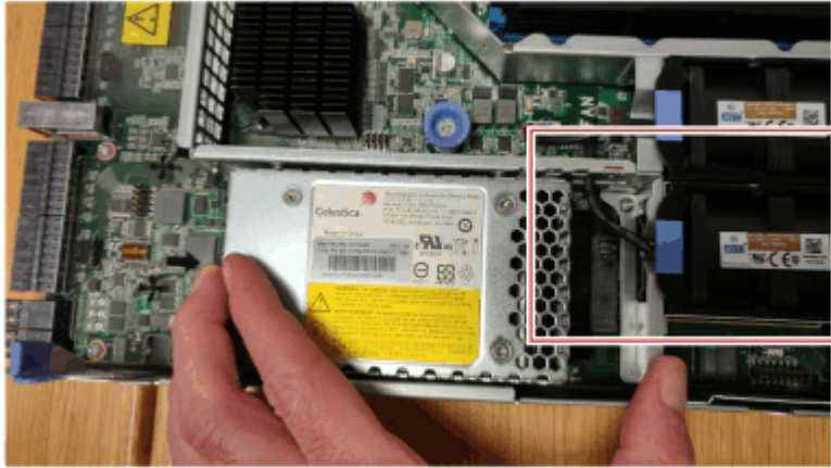
Figure 87. Aligning the cable connector for fan 5
