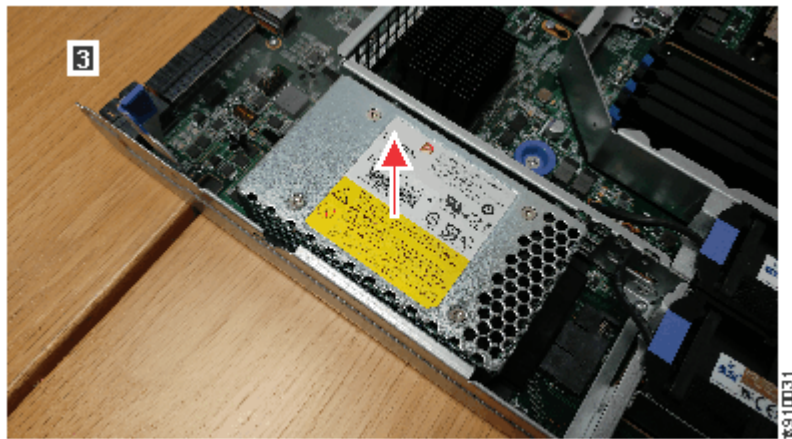
Figure 75. Removing the node battery
