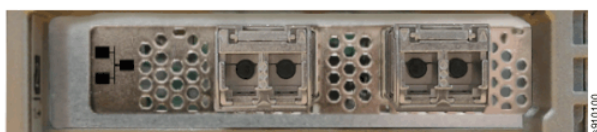
Figure 174. Dual-port 25 Gbps Ethernet host interface adapter ports and LEDs (RoCE)
