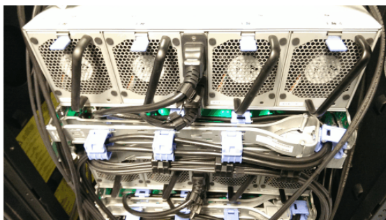
Figure 53. Power and SAS cable connections on the back of the enclosure
