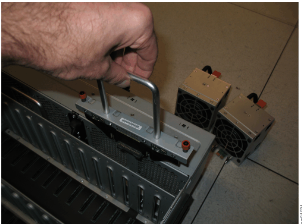
Figure 166. Remove the FIB from the chassis
