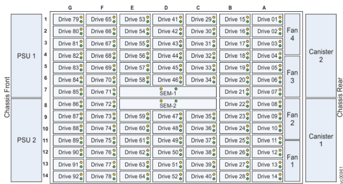
Figure 180. LEDs on drives and SEMs
