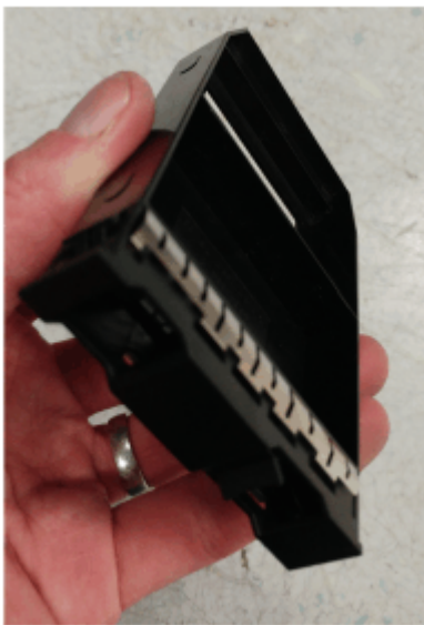
Figure 102. Correct drive blank orientation
