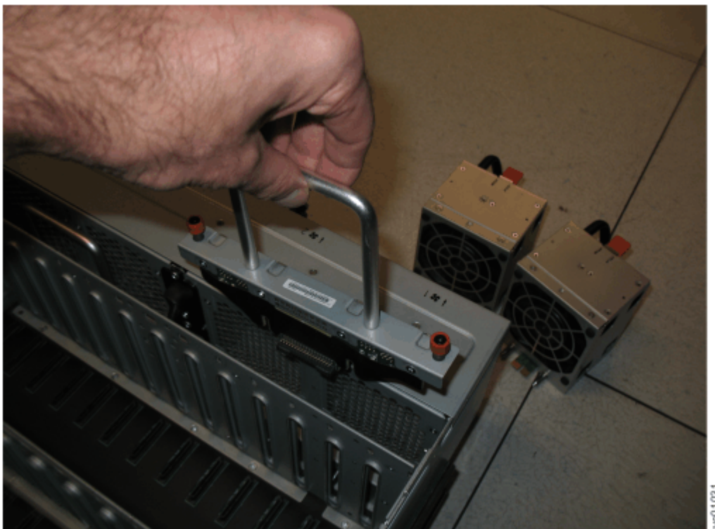
Figure 150. Remove the FIB from the chassis
