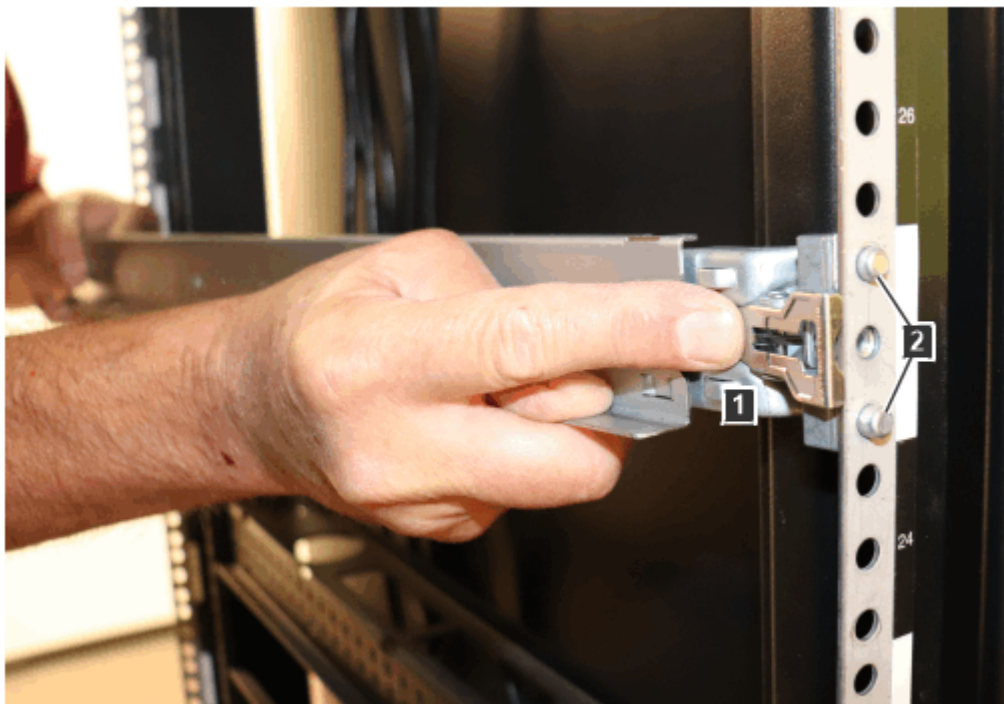
Figure 70. Installing the rear rail bracket
