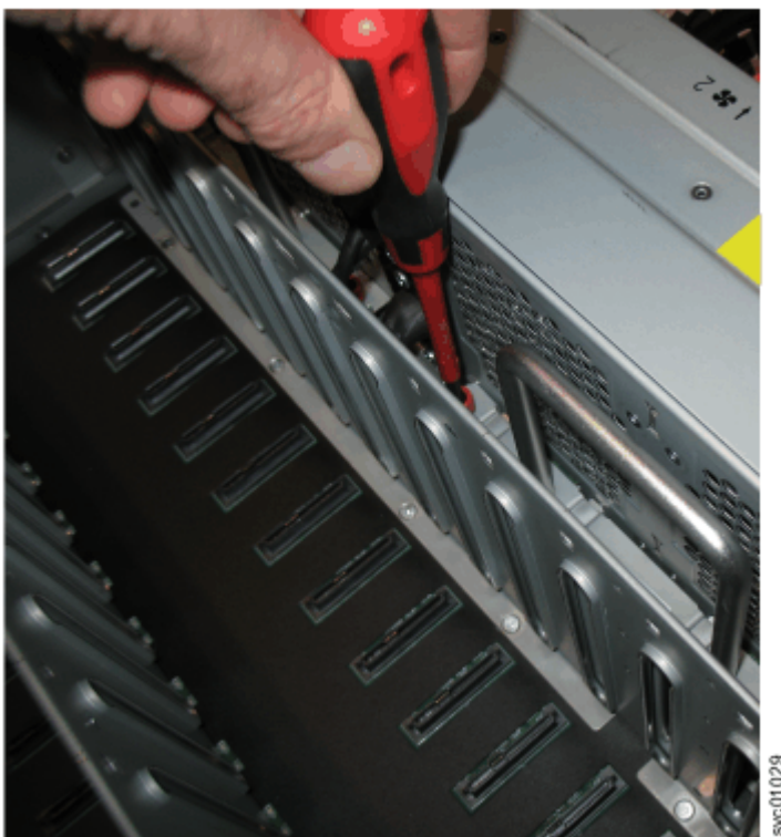
Figure 149. Loosen the FIB screws
