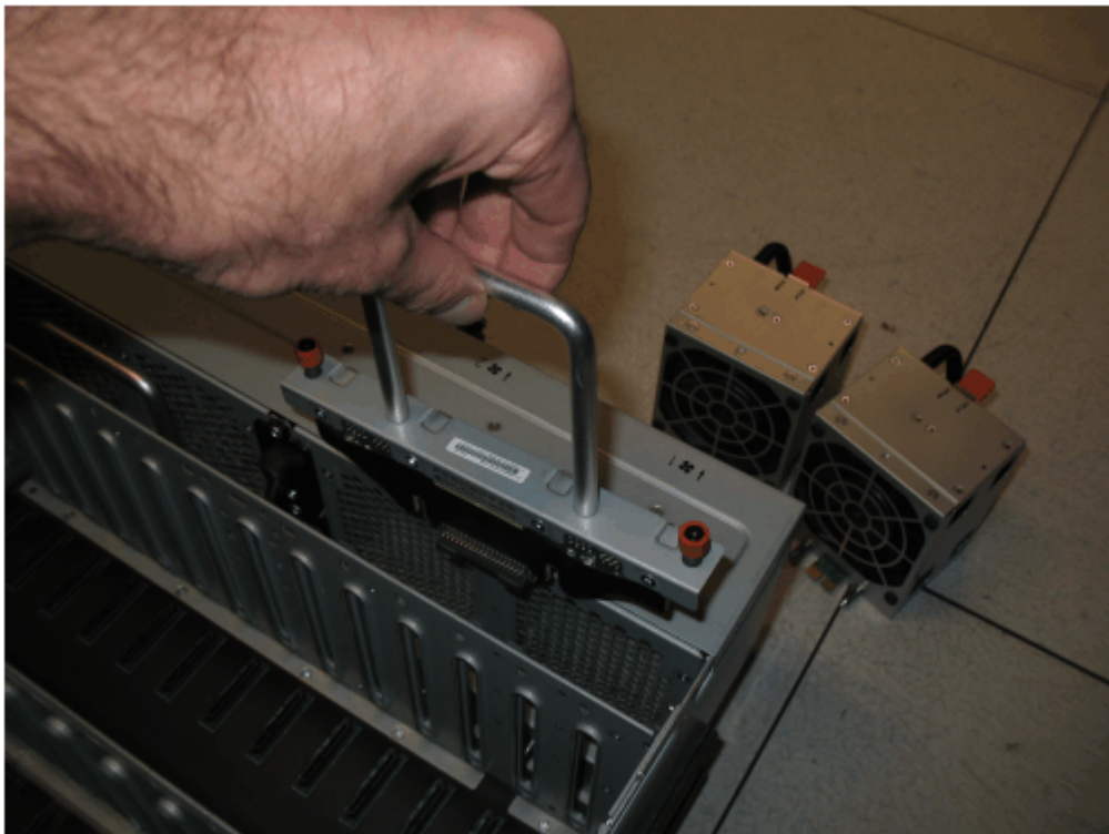
Figure 140. Remove the FIB from the chassis
