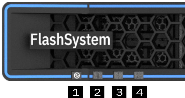
Figure 142. Enclosure health LEDs
