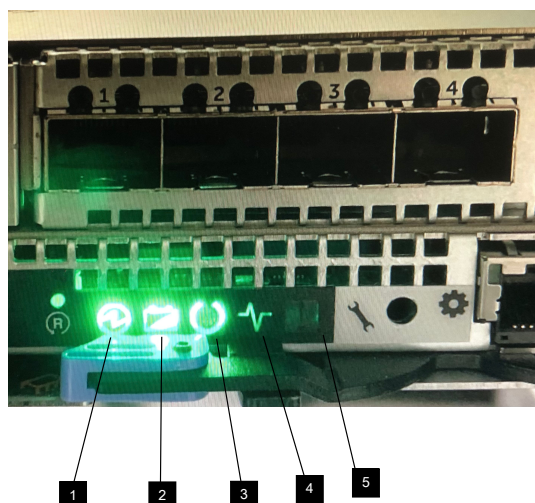
Figure 157. Canister and node status LEDs
