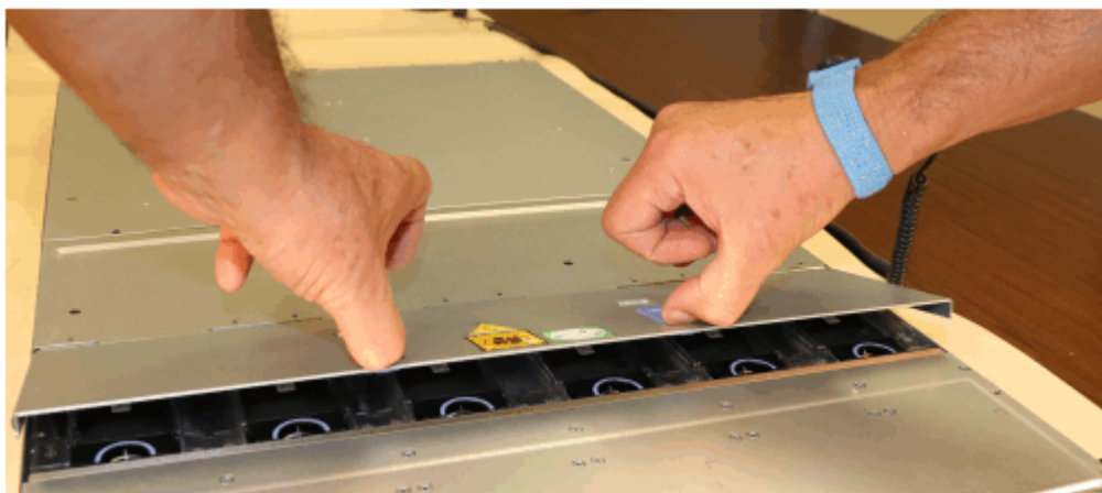
Figure 85. Opening the fan door
