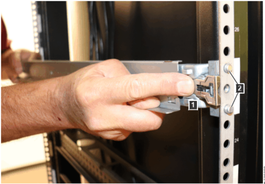
Figure 66. Installing the rear rail bracket
