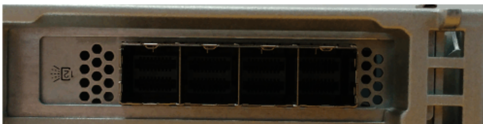
Figure 162. Quad-port 12 Gbps SAS network adapter
