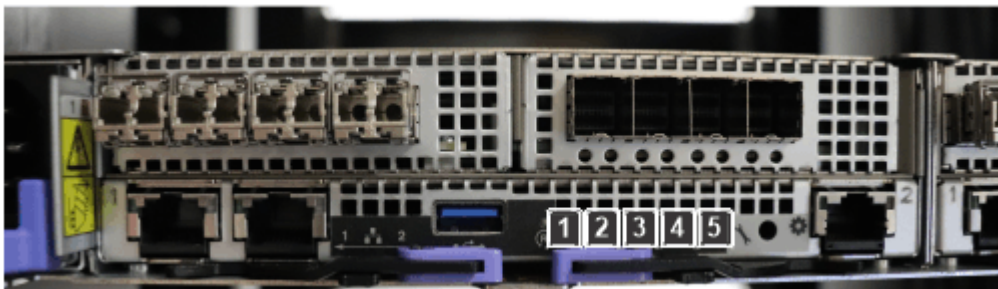
Figure 62. Canister power LED location
