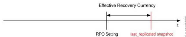
Figure 2. The way RPO_Lagging is determined RPO_Lagging
