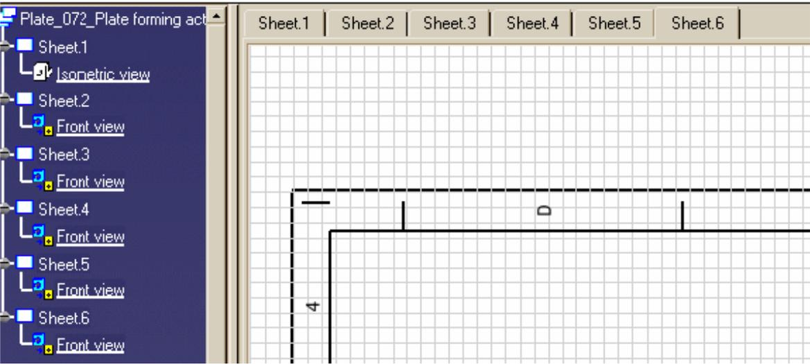
Plus a first sheet showing the isometric view of templates on the curved plate. This sheet has the same viewpoint as the 3D model. If the user changes the viewpoint, for example, rotates the model, then generates the drawing again, the isometric view on the first sheet will be updated to reflect the viewpoint of the 3D model.
