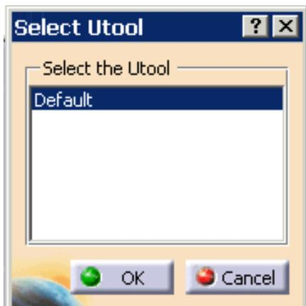
5. Select the Utool (tool profile) if required, and click **OK**. The values for the selected tool profile are displayed in the **TCP Values** dialog box.
