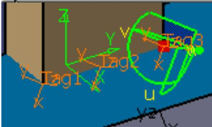
7. Angularity can be stepped up or down 10 degrees using the arrows. To change the step size, change the number of the **Angular Step**.
