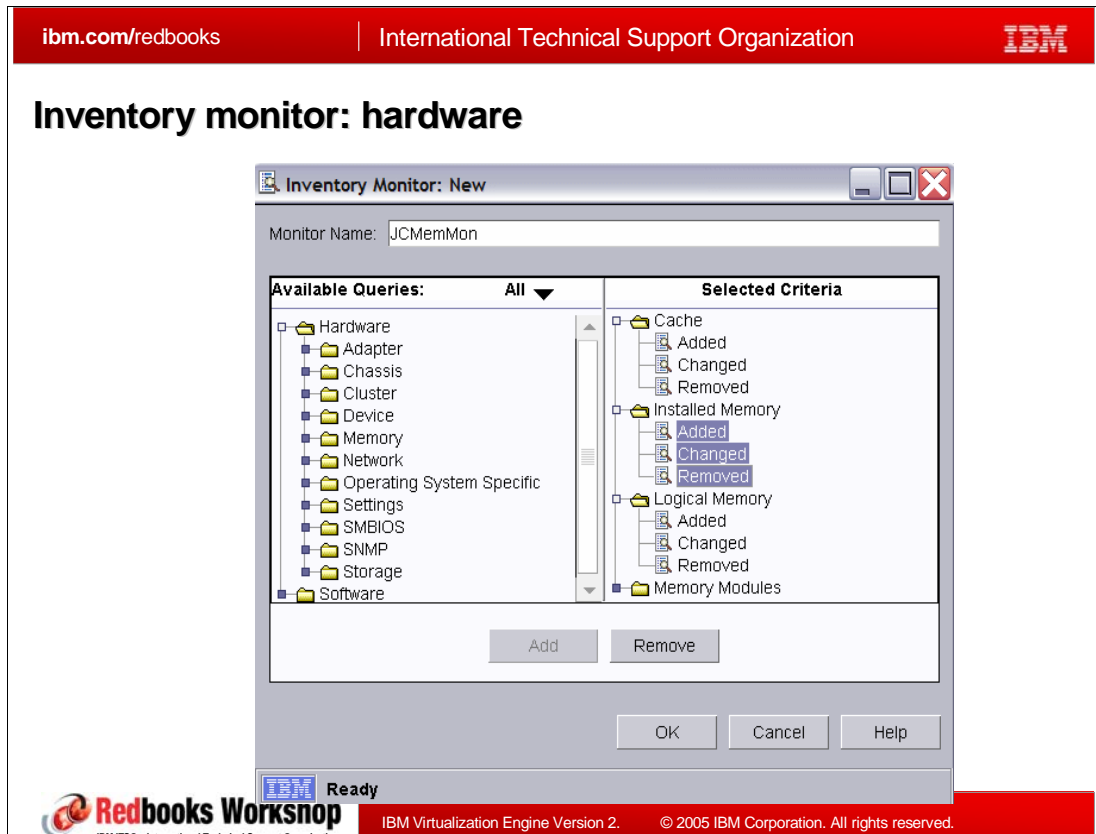
Figure 2-27 Inventory monitor - hardware example
